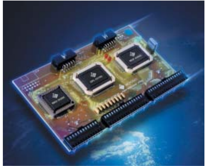
Micronas chips soldered on a PCB for TV audio. Pro Logic II is located in MAS 3529H.
