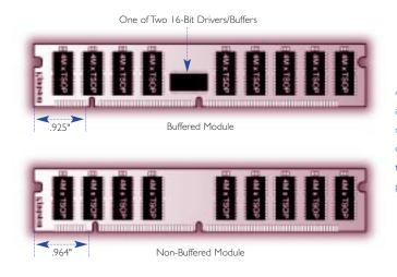
An example of a buffered and a non-buffered module. They are keyed differently, to ensure that they can't be used in place of one another:
