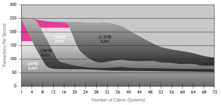
Application servers are utilized to host a wide range of applications, such as word processing and spreadsheet programs. By increasing base memory from 64MB to 256MB, Windows NT Server was able to support five times as many clients before transactions per second dropped.
