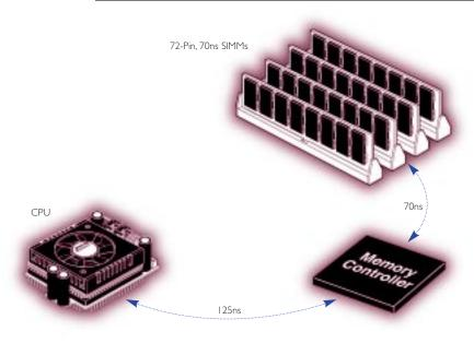
In this example, the memory controller requests data from memory and memory reacts to the request in 70ns.The CPU receives the data in approximately 125ns. So, the total time from when the CPU first requests information to when it actually receives the information can be up to 195ns when using a 70ns memory module. This is because it takes time for the memory controller to manage the information flow, and the information needs to travel from the memory module to the CPU on the bus
