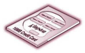
On the surface, credit card memory does not resemble a typical memory module configuration. However, on the inside you will find standard TSOP memory chips.
